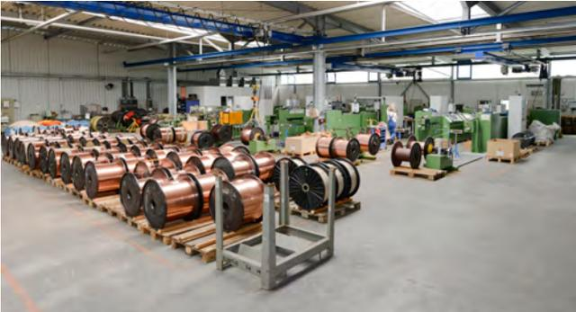
wires. We produce flat wires in all standard dimensions with a variety of insulation types. Apart from the manufacture and insulation of flat wires we dispose of yarn-covering systems for round wires that allow finishing bare or enamelled round wires with different types of insulations.
