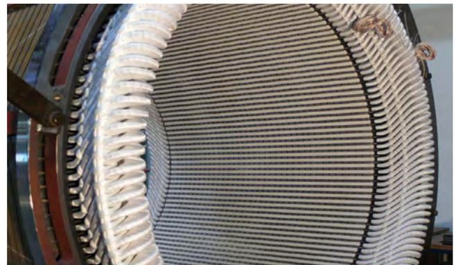
Stator with preformed coils and mica-film insulated wire
