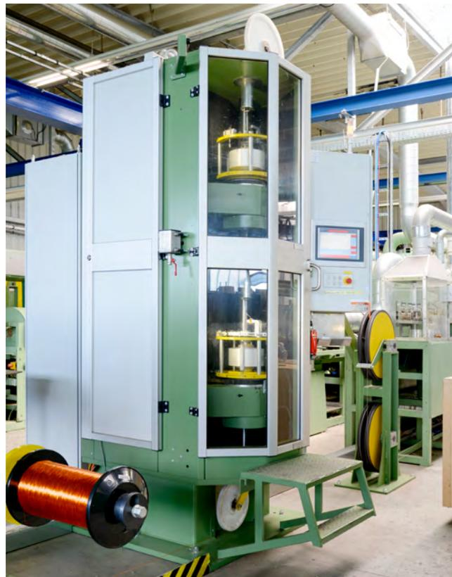
Glass fibre and blended yarn insulation line
