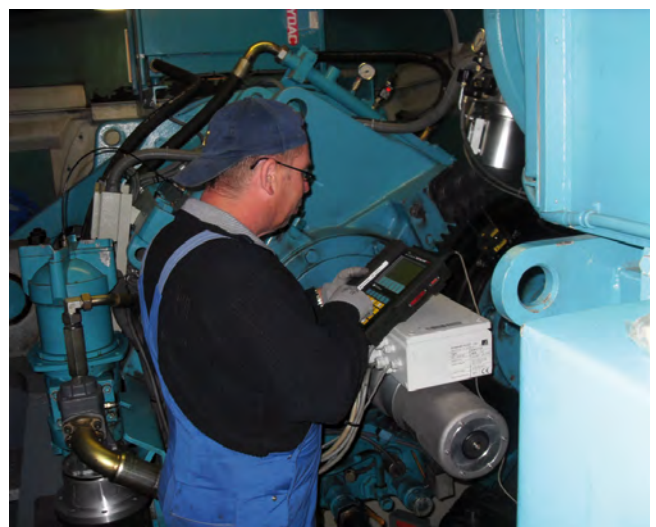
Laser-optical alignment control measurement
